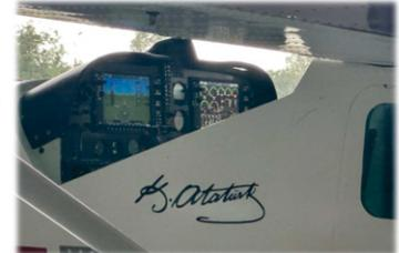
The Turk MFI-17 has an advanced Garmin federated dual screen Glass Cockpit, a crash survivable Flight Data Recorder (black box); an integrated DME, full function Engine, Airframe and Fuel Information system; and support electronics to comply with EASA/FAA 23 civil certification requirements.
